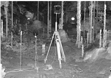
Fig. 3. Ultrasonic anemometer in Katerinska cave. Photo: Jiří Hebelka
