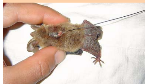
Bechstein's bat with a transmitter LB-2 (0.52 g). The transmitter is attached to the fur of the bat's back with a natural rubber adhesive and the battery lasts for 21 days
