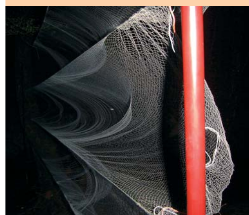
Telescopic fishing poles without drivers are the best for setting mist-nets
